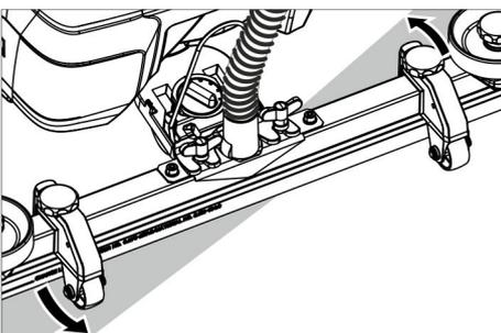
→ Tighten the wing screws.
