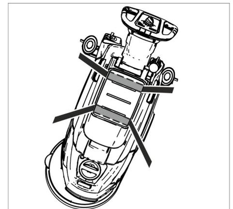
→ When transporting in vehicles, secure the appliance according to the guidelines from slipping and tipping over.
