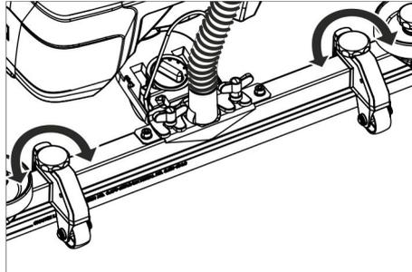
→ Try adjusting the twist handles of the height adjustment until the best vacuuming result is achieved.
