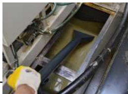
Sludge removal from CNC collection tanks
